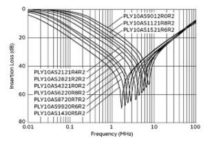
Differential Mode Insertion Loss (Typ.)
