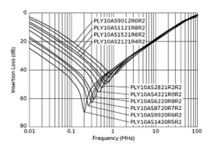
Common Mode Insertion Loss (Typ.)
