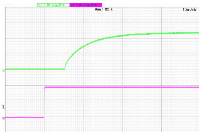
Turn-on transient at full load current (10ms/div). Top Trace: Vout; 2V/div; Bottom Trace: ON/OFF input: 5V/div.
