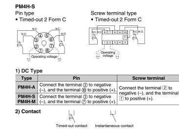
3) Voltage should not be applied to the various inputs (reset, start, and stop) of the PM4H-A multi-range timer. These inputs should be input without voltage.
