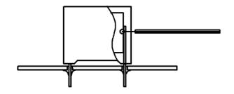
Temperature monitored inside the capacitor.
