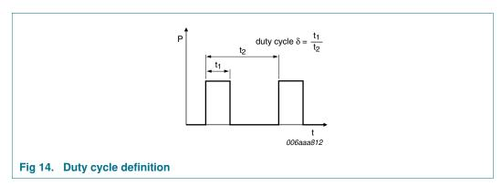
The current ratings for the typical waveforms as shown in Figure 9, 10, 11 and 12 are calculated according to the equations:  $I_{F(AV)} = I_M \times \delta$  with  $I_M$  defined as peak current,  $I_{RMS} = I_{F(AV)}$  at DC, and  $I_{RMS} = I_M \times \sqrt{\delta}$  with  $I_{RMS}$  defined as RMS current.
