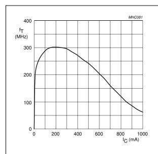
NPN transistor;  $V_{CE} = 10 \text{ V}.$
