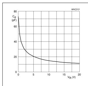
Schottky barrier diode; f = 1 MHz;  $T_{amb} = 25 \,^{\circ}\text{C}$ .
