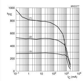
NPN transistor;  $V_{CE} = 5 \text{ V}.$
