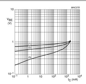
NPN transistor;  $V_{CE} = 5 \text{ V}.$
