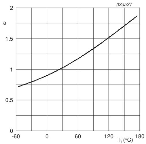
$$a = \frac{R_{DSon}}{R_{DSon(25^\circ\text{C})}}$$
