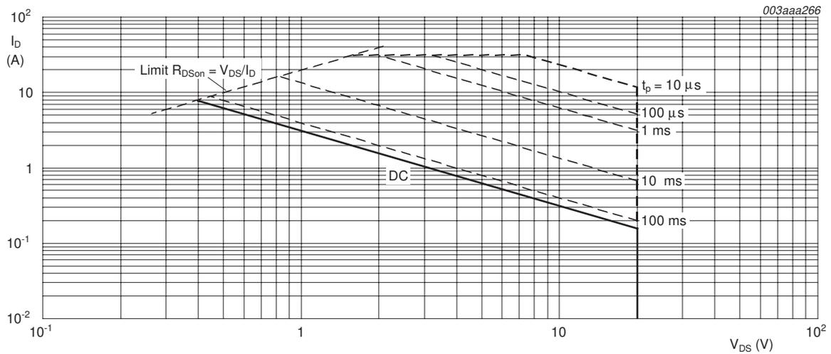
$T_{sp} = 25^\circ C$ ;  $I_{DM}$  is single pulse
