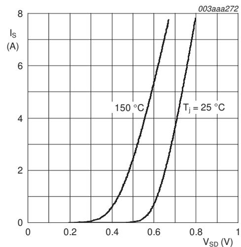
$T_j = 25 \text{ }^{\circ}C \text{ and } 150 \text{ }^{\circ}C; V_{GS} = 0 \text{ V}$
