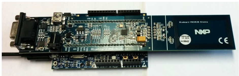
Fig 14. CLEV663B connected to LPCXpresso LPC11U68 development board
