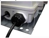
(must comply with all local, national and country electrical codes) from source through piping/gland to the terminal block. The AC cable will need to be a minimum of 14AWG and terminated with M3.5 spade lugs. Pair and secure ground, line, and neutral to the appropriate positions on the three pin terminal block and reattach the protective covering. Note: if using the cable gland PGLAND750, the outer seal nut needs to be fully tightened to close rubber seal to protect against ingress of water.
