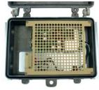
Connect cable glands (PGLAND750) or ¾ NPT conduit piping to the face of the midspan. Ensure that connectors are fully installed to guarantee waterproof operation.
