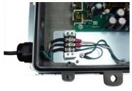
6) Using waterproof outdoor rated Cat5e Ethernet cable, thread through cable glands or conduit piping to the appropriate RJ45 connector and ensure each portal is properly sealed.
