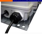
(must comply with all local, national and country electrical codes) from source through piping/gland to the terminal block. The AC cable will need to be a minimum of 14AWG and terminated with M3.5 spade lugs. Pair and secure ground, line, and neutral to the appropriate positions on the three pin terminal block and reattach the protective covering. Note: if using the cable gland PGLAND750, the outer seal nut needs to be fully tightened to close rubber seal to protect against ingress of water.
