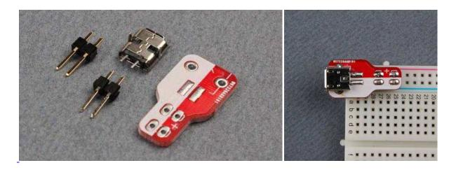
Breaking out a nifty little power only micro-b USB connector it will deliver a very usable 5V to a single power rail on your breadboard.
