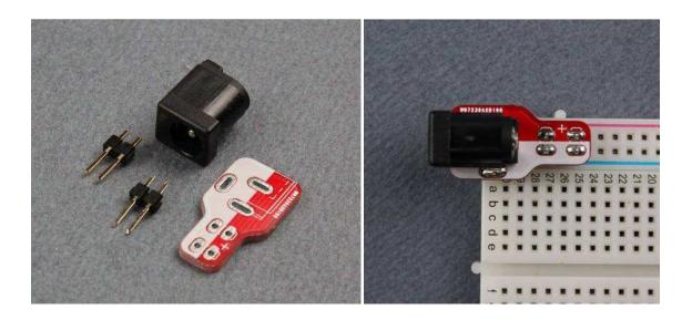
This simple little kit takes moments to solder but will make your bread-boarding life a whole lot easier for years to come. Breaking out a DC barrel jack connector it will deliver whatever power your PSU is rated for to your breadboards power rail.
