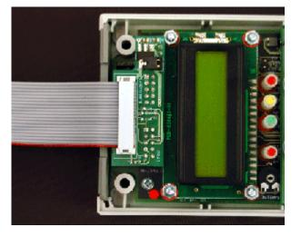
A special AT91SAM7 ISP cable has been developed which connects between an Equinox portable ISP programmer and any SAM7 Target System.
