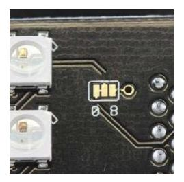
WARNING: These little WS2812B Neopixel fellas can get VERY bright so we recommend running at a low brightness ONLY (we recommend 1/8th which is 32 out of 255 in your code). If you run the micro:pixel board at brightnesses higher than this, then you may well damage your micro:bit board as the pixels will try to pull more power than the micro:bit itself can handle.
