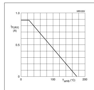
Fig.2 Maximum average forward current as a function of ambient temperature.
