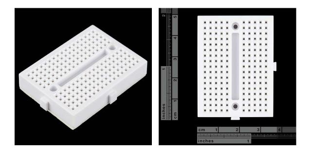
**Description:** This white Mini Breadboard is a great way to prototype your small projects! With 170 tie points there's just enough room to build and test simple circuits; They're also great for breaking out DIP package ICs to jumper wires! If you run out of room, no worries, these mini breadboards can be snapped together to form larger stretches of board. It has a peel and stick adhesive backing as well as two mounting holes for M2 screws so you can anchor it down.
