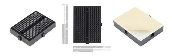
**Description:** This black Mini Breadboard is a great way to prototype your small projects! With 170 tie points there's just enough room to build and test simple circuits; They're also great for breaking out DIP package ICs to jumper wires! If you run out of room, no worries, these mini breadboards can be snapped together to form larger stretches of board. It has a peel and stick adhesive backing as well as two mounting holes for M2 screws so you can anchor it down.
