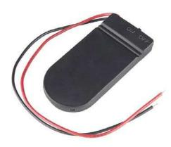
**Description:** This is a simple coin cell battery holder that can enclose two CR2032 batteries inside itself, and safely kept closed via two phillips head screws. Each battery holder will run batteries in series, output up to 6V, and is equipped with an On/Off slide switch and two 6" power wires (one positive and one negative) on the back.
