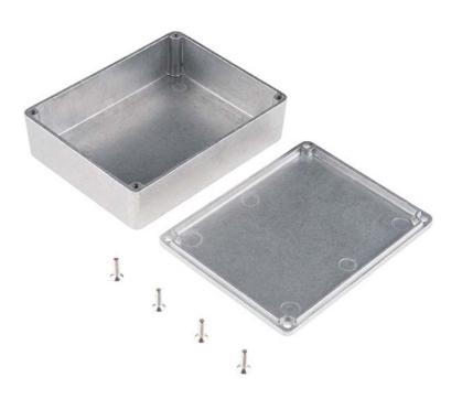
These are our large, beefy aluminum enclosures, which have been built tough enough to withstand a truck. This 2mm-thick, die-cast enclosure is rated IP54 against dust and splashing water. Because it's aluminum, it's easy to cut and drill so that you can add LCD screens, buttons and cable connections. If you want to "pretty up" your project, hit this with some fine-grit sand paper and buff it or just spray paint it!
