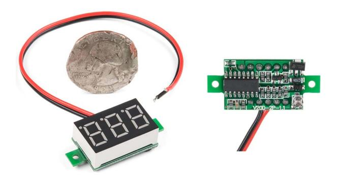
**Description:** This Digital LED Voltmeter measures the voltage at a particular point of the system it has been hooked up to and then provides a readout on its three 7-segment LEDs. This voltmeter is able to provide a readout of voltages from 2.5VDC to 30VDC within a 1% accuracy.
