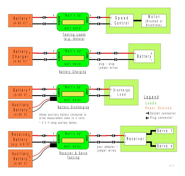
The following are some example **three-wire meter connections**. Many other arrangements and uses are possible.
