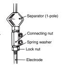
Note: 1. The spring washer comes with the lock nut.
