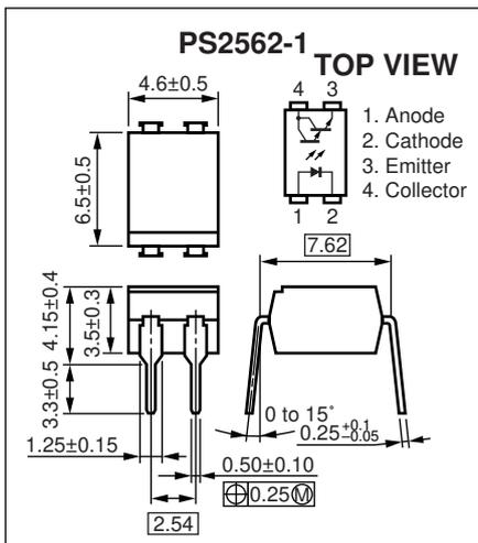
**Lead Bending Type (New package)**
