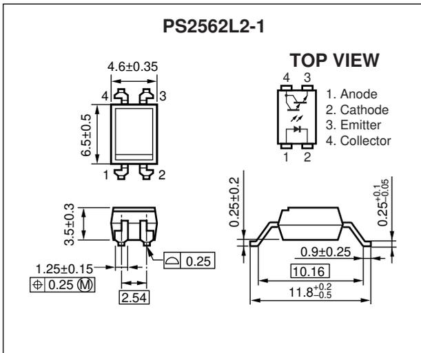
**Lead Bending Type For Long Creepage Distance (Gull-Wing)**
