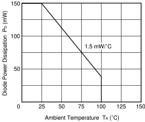
**TRANSISTOR POWER DISSIPATION vs. AMBIENT TEMPERATURE**
