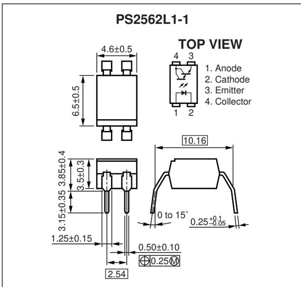
**Lead Bending Type For Long Creepage Distance (Gull-Wing) (New Package)**
