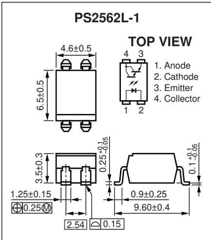
**Lead Bending Type For Long Creepage Distance (New Package)**
