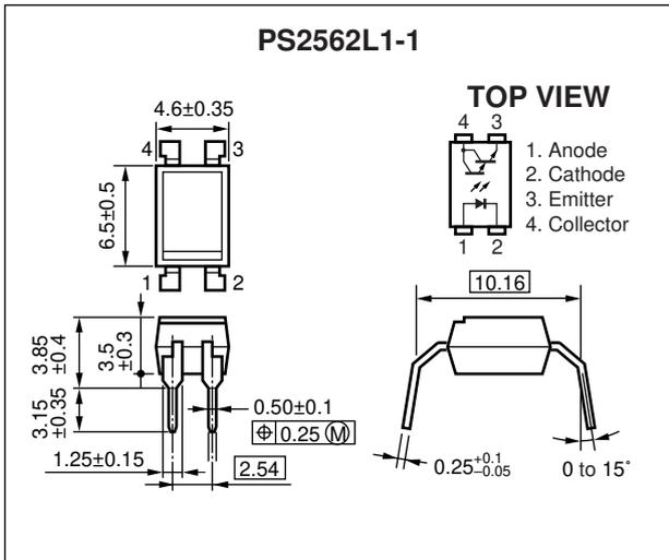
**Lead Bending Type For Long Creepage Distance**
