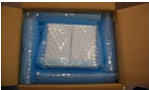
Inner boxes concluding sensors are put into the outer box (210mm × 210mm × 154mm), and fixed by air packing.
