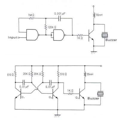
It should be noted that the component values given are starting points only. For example, the inductor shown is optional and the value of the inductor will definitely have to be adjusted depending on the transducer used. Also, the oscillator portion of the transistor circuit will have to be adjusted to match the resonant frequency of the transducer.
