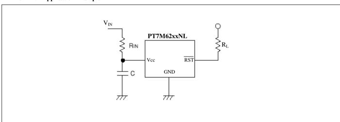
Please use N-ch open drains configuration, when a resistor  $_{RIN}$  is connected between the  $V_{CC}$  pin and power source  $V_{IN}$ . In such cases, please ensure that  $R_{IN}$  is less than  $10k\Omega$  and that C is more than  $0.1\mu F$ .  $R_L$  could be  $1k\Omega$  to  $510k\Omega$ .
