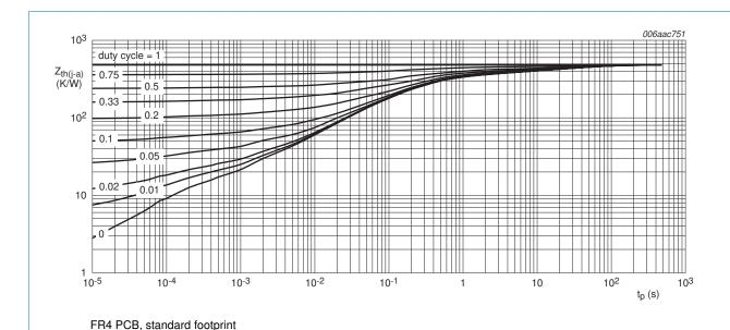
Fig 2. Transient thermal impedance from junction to ambient as a function of pulse duration for PEMD3 (SOT666); typical values
