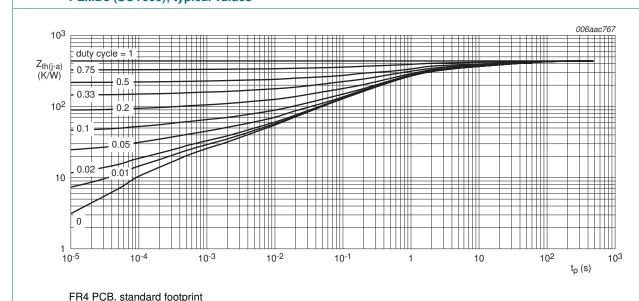
Fig 3. Transient thermal impedance from junction to ambient as a function of pulse duration for PIMD3 (SOT457); typical values
