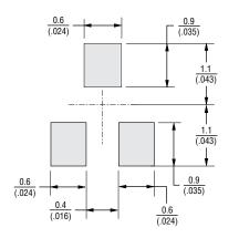
$\begin{array}{l} \text{DIMENSIONS: } \displaystyle \frac{\text{MM}}{(\text{INCHES})} \\ \text{TOLERANCES: } \pm \displaystyle \frac{0.1}{(.004)} \\ \text{EXCEPT WHERE NOTED} \end{array}$
