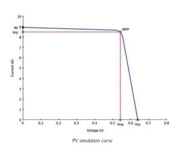
The PVS power supply outputs points on the I-V curve in 1 ms intervals to test the inverter's MPPT efficiency.
