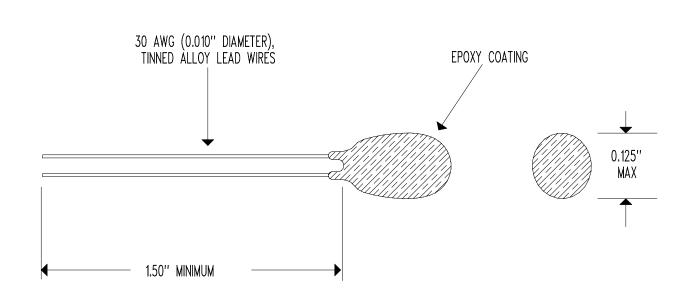
RESISTANCE @  $+25^{\circ}C$  = 1,000  $\Omega$  NOMINAL ACCURACY (0 TO  $+70^{\circ}C$ ) =  $\pm$  0.50°C RESISTANCE/TEMPERATURE CURVE = "J" TEMPERATURE COEFFICIENT @  $+25^{\circ}C$  = -4.4%/°C NOMINAL BETA " $\beta$ " (0 TO  $+50^{\circ}C$ ) = 3,892°K NOMINAL DISSIPATION CONSTANT = 1 mW/°C NOMINAL THERMAL TIME CONSTANT = 10 SECONDS MAXIMUM (STILL AIR) THERMAL TIME CONSTANT = 1 SECOND MAXIMUM (WELL STIRRED OIL) MAXIMUM TEMPERATURE RATING =  $+150^{\circ}C$
