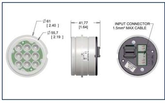
Diameter x H 61mm x 41.8mm (2.40" x 1.65") Maximum Cable Dia - 1.5mm<sup>2</sup> / 16 AWG
