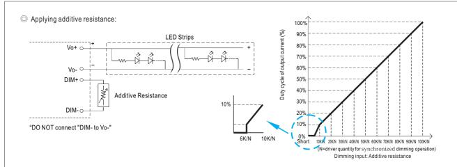
Note: 1. Min. duty cycle of output current is about 6% and the output current is not defined when 0% < Iout < 6%.
