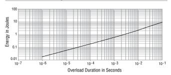
The energy absorbed by the resistor expressed in Joules can be calculated by multiplying the peak power of the pulse in watts times the length of the pulse in seconds.
