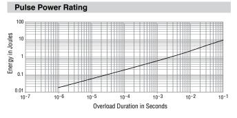
The energy absorbed by the resistor expressed in Joules can be calculated by multiplying the peak power of the pulse in watts times the length of the pulse in seconds.
