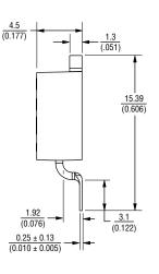
MM DIMENSIONS: (INCHES) ±0.38 TOLERANCE: UNLESS OTHERWISE NOTED (±0.015) 0.102 LEAD MAX AT MOUNTING COPLANARITY: (0.004) SURFACE
