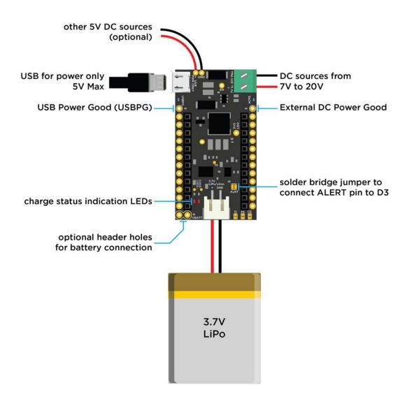
There are two status LEDs located on the left of the JST battery connector labeled STAT1 and STAT2. Here is a table of the LED behavior depending on which state the battery charger is in:
