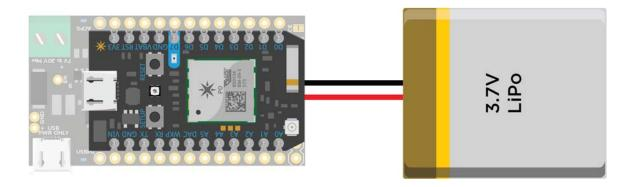
The shield is setup so that when powered from the USB port as well as from a DC supply, it chooses the DC source over USB. The charge current is set to 500mA when charging from USB and set to 1A when charging from a DC source.
