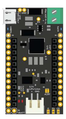
The system switches in between the different power sources automatically, reducing the charge and discharge cycle stress on the battery. The fuel gauge allows you to monitor the battery's state-of-charge (SOC), allowing it to notify the user remotely and take preemptive actions when necessary.
