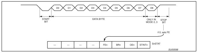
Figure 13. UART Framing Error Detection
