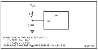
Figure 15. Recommended Reset Circuit
