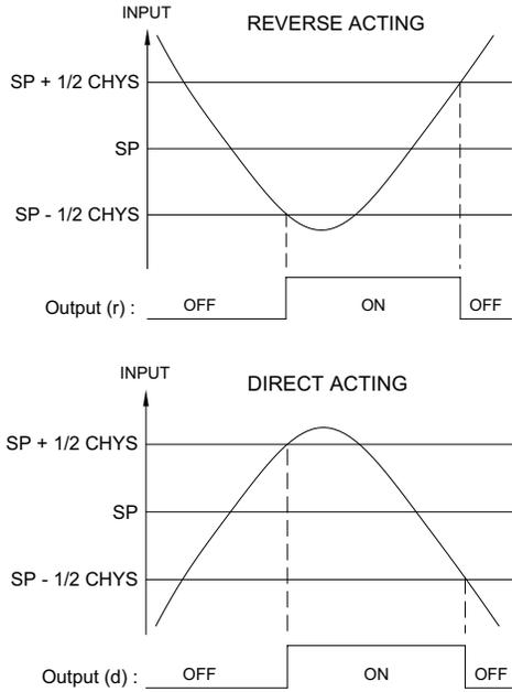
Note: CHYS in the On/Off Control Figures refers to the On/Off Control Hysteresis (CHYS) in parameter Module 2.
