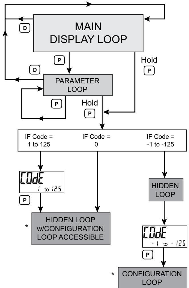
\* If PLOC is active, the Configuration Loop is not accessible.
