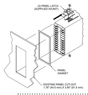
The controller is designed to be mounted into an enclosed panel. The unit must be inserted in the case during installation of the controller.
