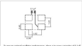
To ensure optimal oscillator performance, place a by-pass capacitor of  $0.1\mu F$  as close to the part as possible between Vdd and GND pads.
