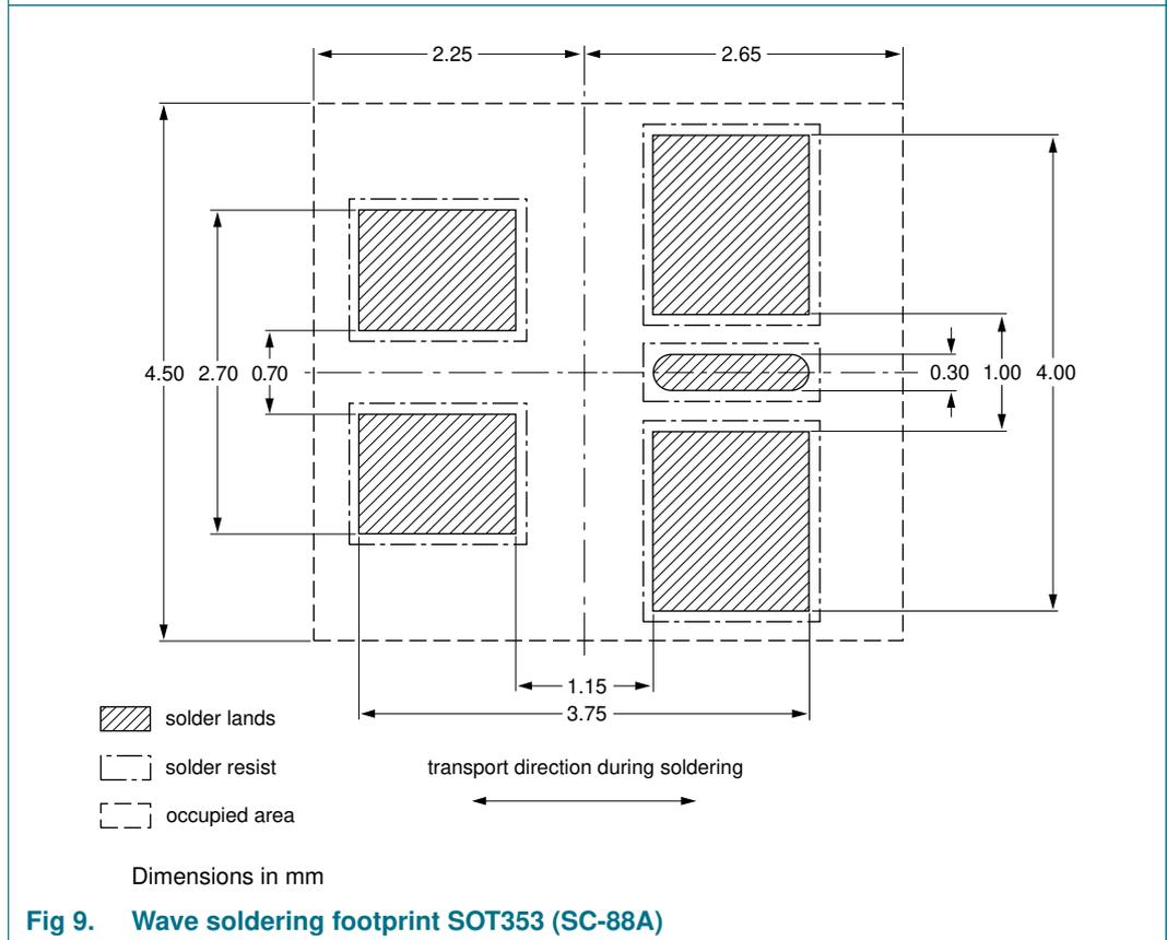
Fig 9. Wave soldering footprint SOT353 (SC-88A)
