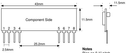
Pins on 0.1" pitch Pin Dims :0.25 x 0.50mm
