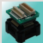
⑥ Target connector Connector soldered onto the target system
