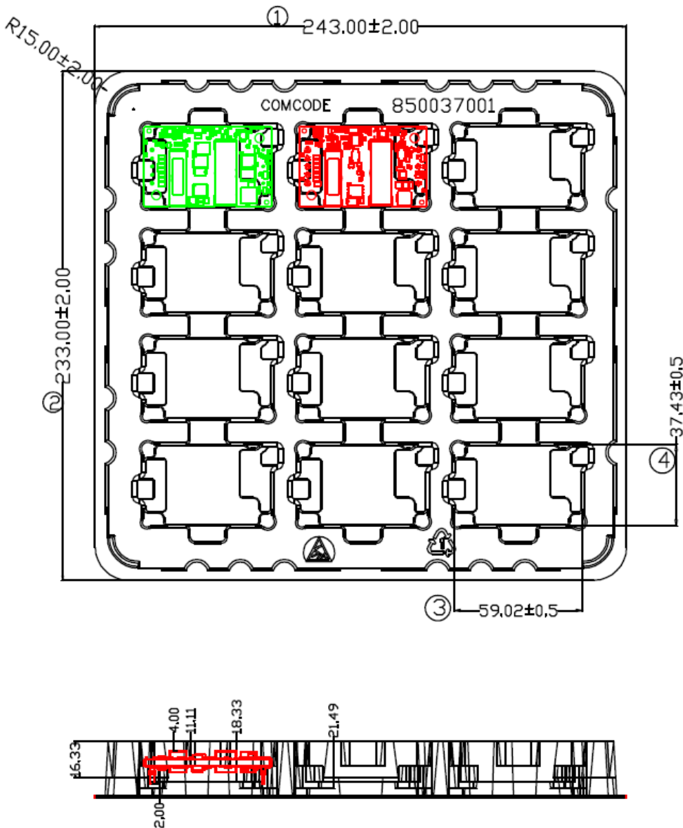
Figure 26. Open Frame Through Hole Packaging Tray
