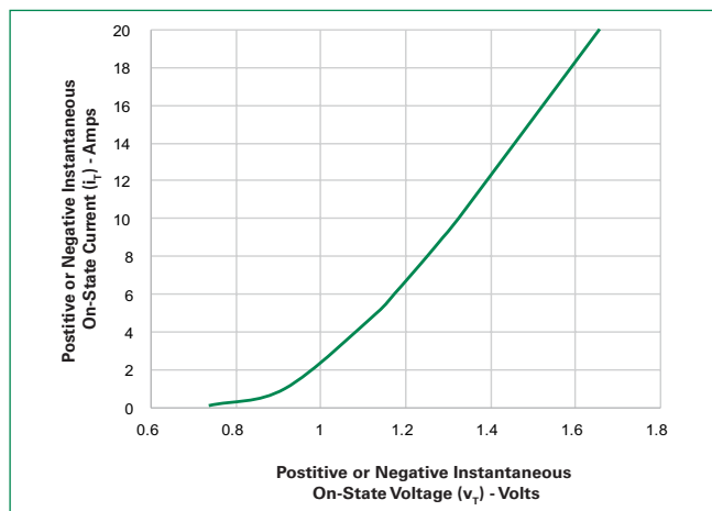
Figure 7: On-State Current vs. On-State Voltage (Typical)
