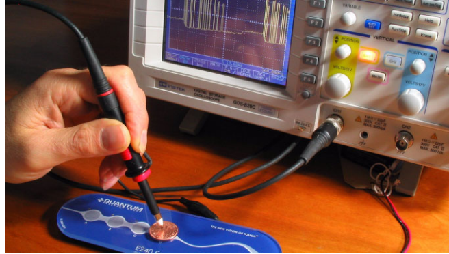
Figure 2-1. Measuring the Charge-transfer Pulses
