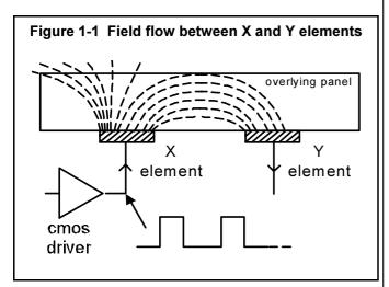
The 60320 uses burst-mode charge transfer methods pioneered and patented by Quantum, including charge cancellation methods which allow for a wide range of key sizes and shapes to be mixed together in a single keypanel. These features permit the construction of entirely new classes of keypanels never before contemplated, such as touch-sliders, back-illuminated keys, and arbitrary shape keypanels, all at very low cost.
