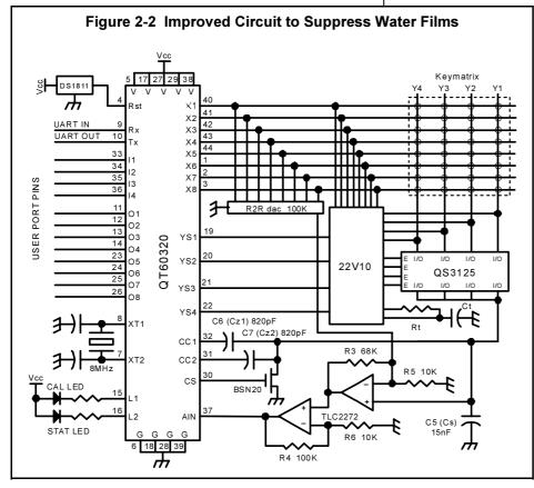
on Cs; each Cz will cancel charge in a discrete step as required.
