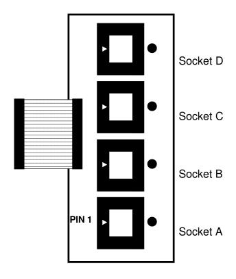
NOTE: Align PIN 1 of 44 pin devices with the arrow indicated.
