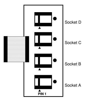
NOTE: Align PIN 1 of 8 pin and 14 pin devices with the arrow indicated.
