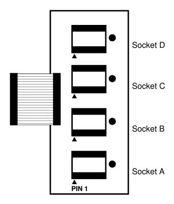
NOTE: Align PIN 1 of 18 pin devices with the arrow indicated.
